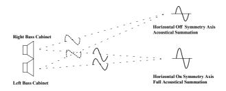
Fig. 8. Two bass cabinets placed side-by-side. Only small travel distance differences for low frequencies
