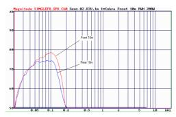
Fig. 1. Frequency response of a typical 18" vented cabinet. Measurement shows front vs rear radiation. Crossover frequency 124Hz, Linkwitz-Riley 24dB/Oct.
