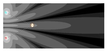
Fig. 7. 'Bass Alleys'. Two bass cabinets with 10m distance. Horizontal coverage at 100Hz
