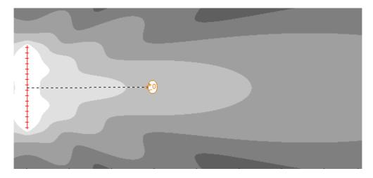
Fig. 13. Horizontal bass array with 16 cabinets, width approximately 10m, horizontal coverage at 100Hz
