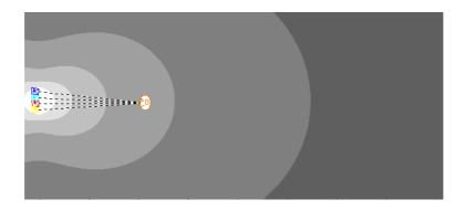
Fig. 11. 1-by-4 Array horizontal coverage at 100Hz. Four 90cm\*60cm bass cabinets side-by-side
