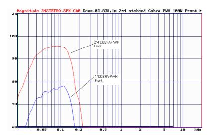
Fig. 16. Comparison of the frequency response of a single 18" vented cabinet vs an array of 2\*4 cabinets.
