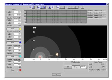
Fig. 3. SPL and directivity of an omnidirectional point source without any reflecting surface, 100Hz
