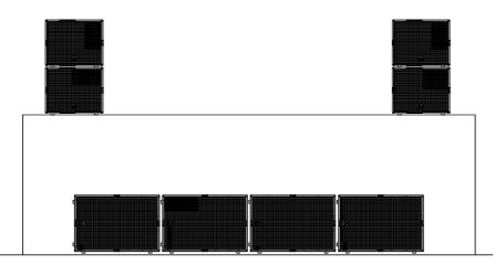
Fig. 12. 1-by-4 Bass array together with mid-high cabinets on stage
