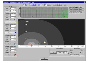
Fig. 4. Ground-stacked bass cabinet with mirrored cabinet, 100Hz
