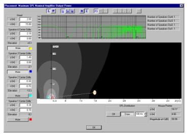
Fig. 5. Idealized cabinet with 70 cm depth placed against a wall at 100Hz (shown with mirror cabinet)
